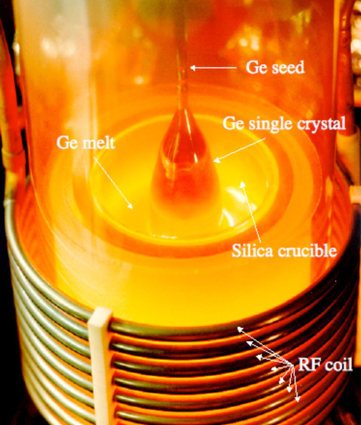
An ultra-pure Germanium single crystal is being “pulled” from a melt contained in a silica crucible at 936°C. The atmosphere is pure Hydrogen. Heat is supplied by the water cooled radiofrequency (RF) coil surrounding the silica envelope. This bulk crystal growth technique carries the name of it’s inventor, “Jan Czochralski .”
