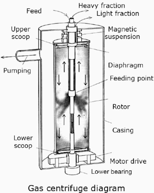
Fig. 6. Principle of gas-centrifuge isotope separation (G.Yu. Grigoriev, 2003).
