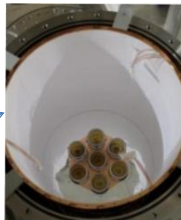
Cu cylinders with WLS foil
