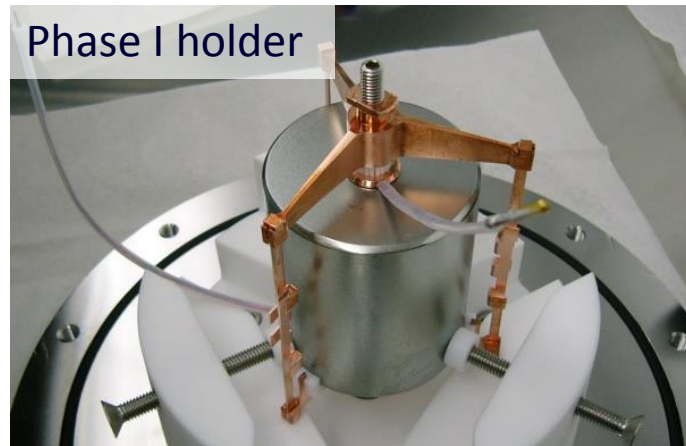
Low mass holder made of ultrapure materials: low-activity Cu (80 g), PTFE, Si
