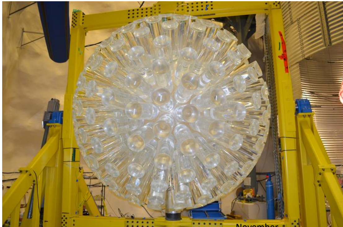
In several passes, stubs are precision machined out of the main AV sphere.
