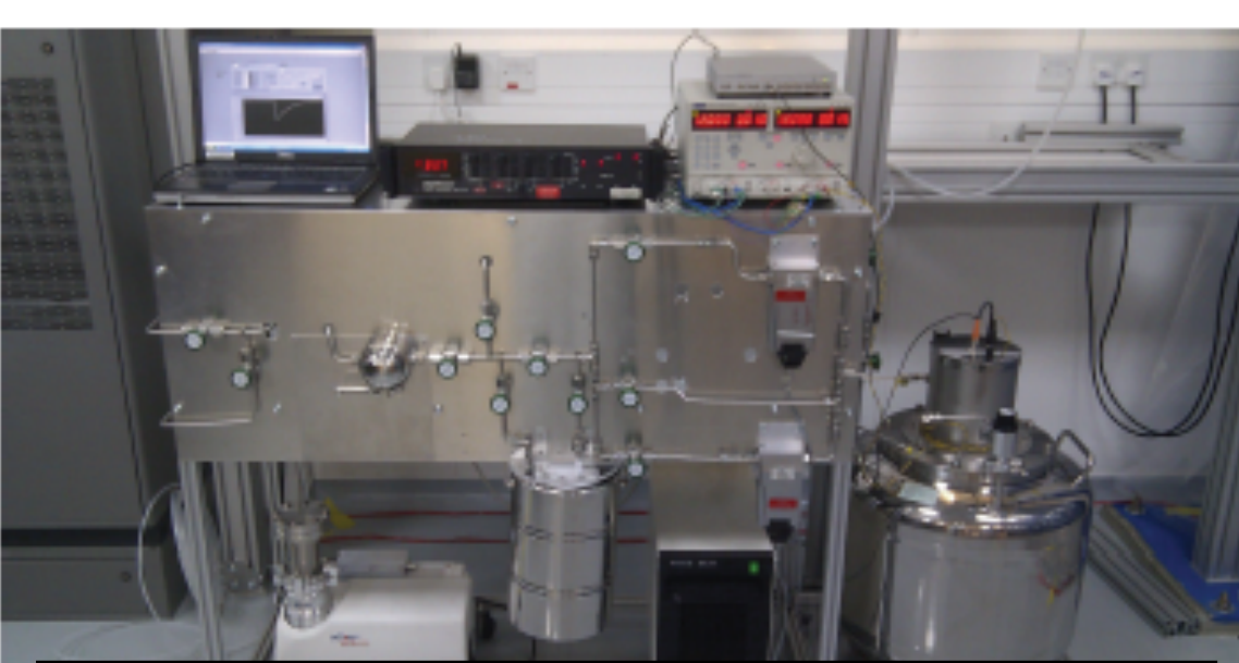
Rn concentration line. Emanation 90uBq/sample large gas volumes \sim 5\text{uBq/m}^3 (UCL-MSSL)
