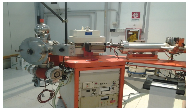
Finnigan MAT 261/262 Thermal Ionization MS Multicollector detector (precise Isotope analysis)
