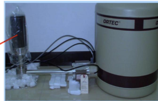
Ortec GEMMX-941000 low bkgd, HPGe Detector used to screen radioactivity of detector components
