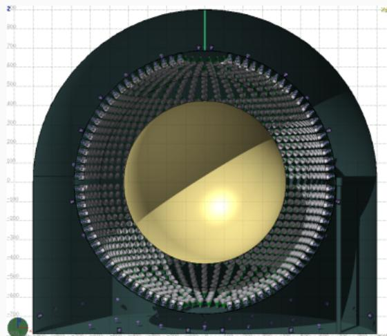
The Borexino inner detector as it was filling up with liquid scintillator and the experiment as it was implemented in FLUKA. Borexino contains approximately 300 t of liquid scintillator in a 8.5 m diameter inner nylon vessel.
