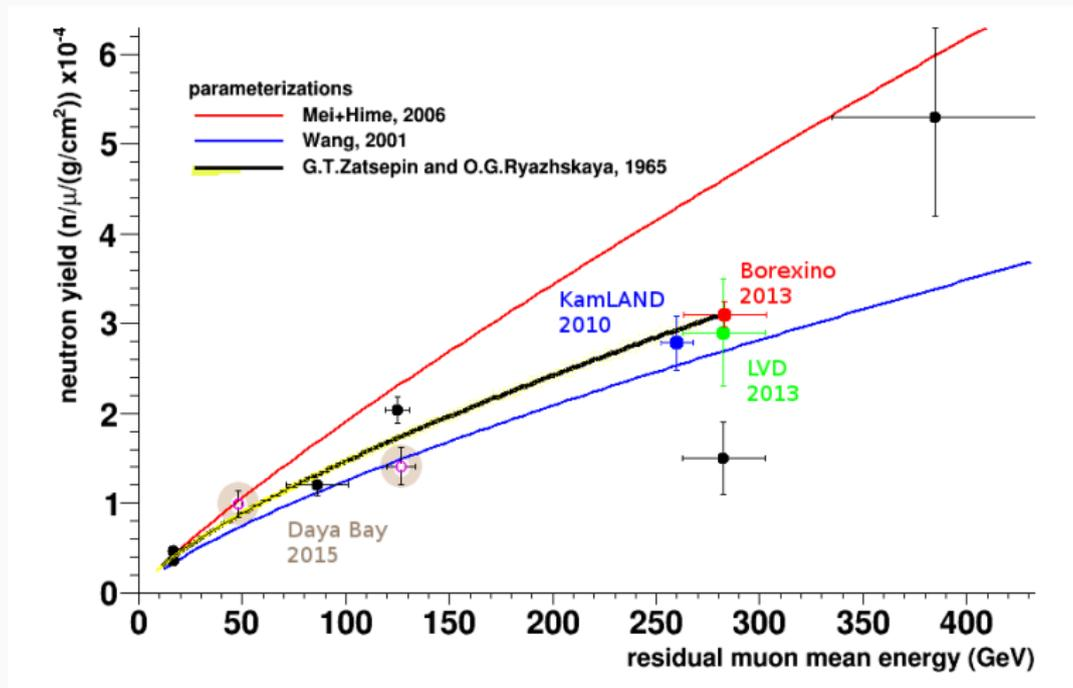
Symbols show the experimental muon-induced neutron yield as originally published. References for data points are given in [JCAP 08 \(2014\) 064 - arXiv:1406.6081](#) except for Daya Bay data points; University of Houston thesis at this point in time
