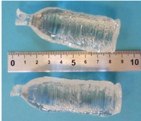
W-doped \text{ZnMoO}_4 grown by LTG Cz
