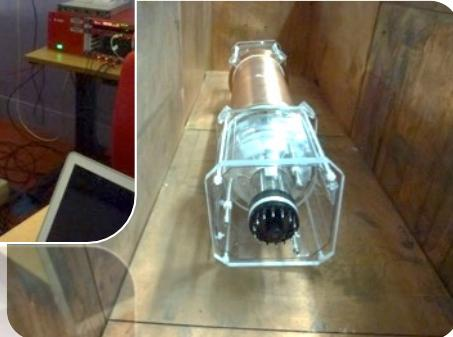
**STATUS:** ULB NaI (Tl) detector array assembly, characterisation & operation prior to installation at the South Pole.
