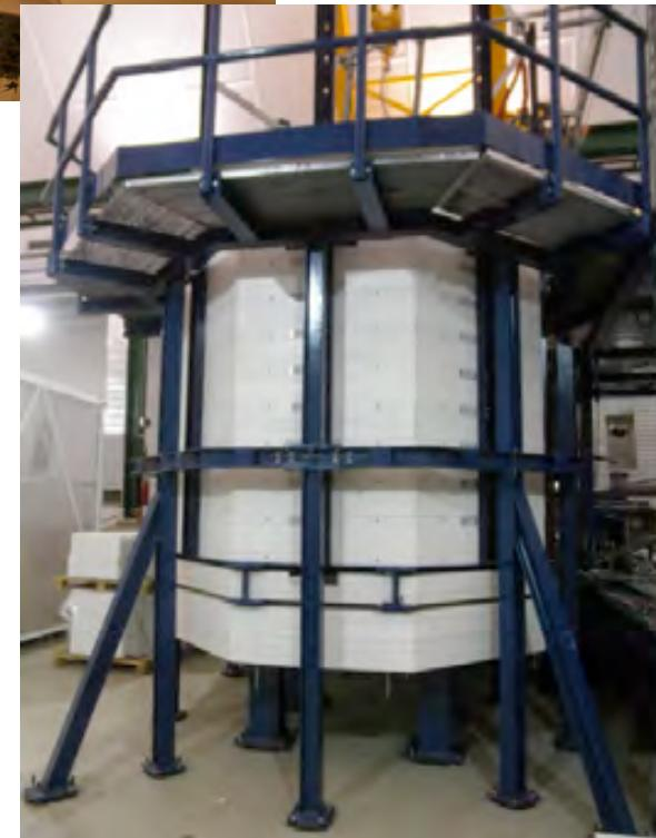
LSC ordered to Alpha Spectra a NaI(Tl) prototype aiming to 20 ppb or less of  $^{40}\text{K}$  Traveling (on surface) to LSC.
