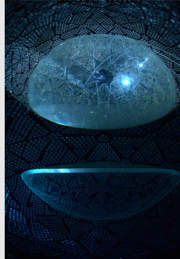
*The detector and cavity are currently about half filled with water.*
